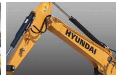
Standard breaker piping
